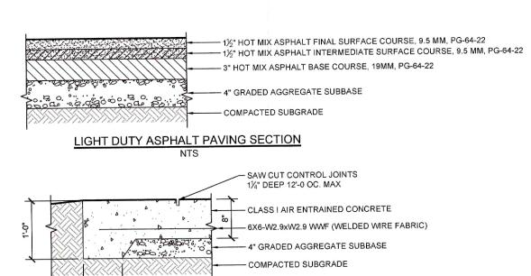
PLACE EXPANSION JOINTS BETWEEN CONCRETE SLAB AND ALL CURBS, BUILDING WALLS, COLUMNS, FOOTINGS, MANHOLES AND CLEANOUTS AND ELSEWHERE AS SHOWN ON PLAN HEAVY DUTY CONCRETE PAVING SECTION
