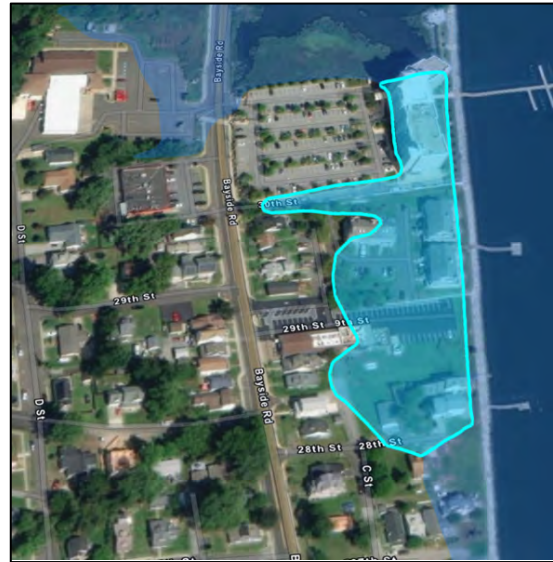
Figure 8: FEMA Flood Zone AO. The base flood elevation may be less than 4 feet but is not mapped by FEMA.
