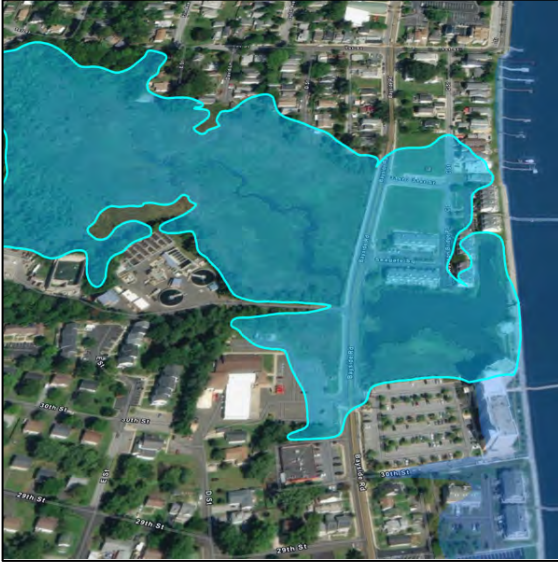
Figure 9: FEMA Flood Zone AO. Base flood elevation is 4 feet.
