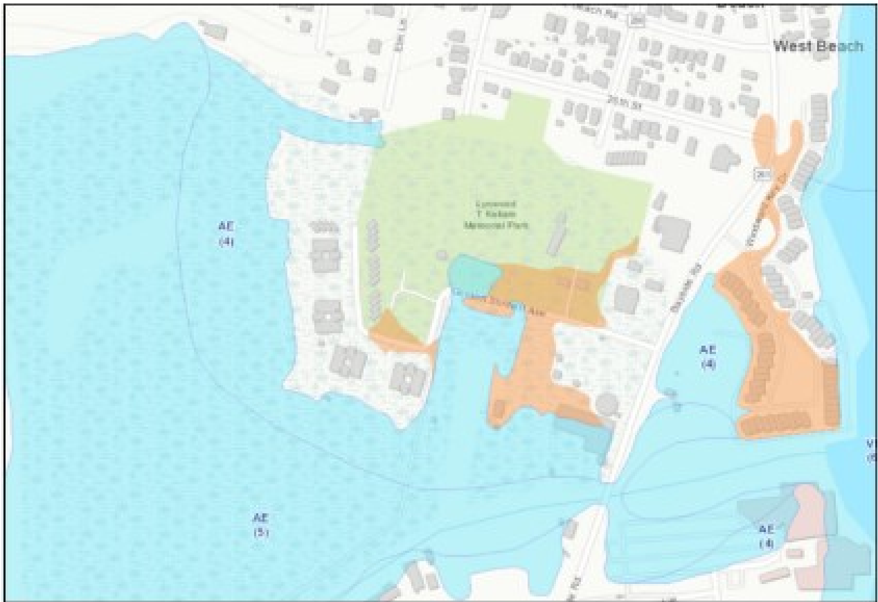
Figure 4: Historic FEMA floodplain mapping showing the extent of the marsh associated with Fishing Creek.
