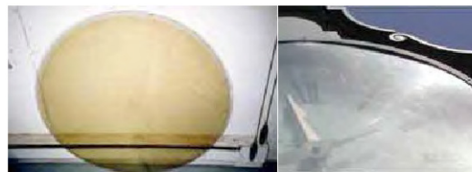
Left - aged LEXAN™ crystal removed during clock renovation. Right - warped & scratched LEXAN™ crystal.
