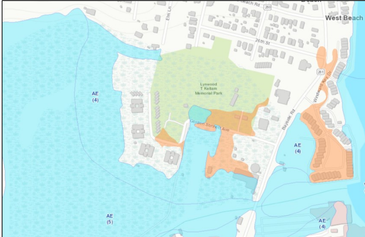
Figure 4: Historic FEMA floodplain mapping showing the extent of the marsh associated with Fishing Creek.
